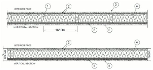
1. **Framing Members\*** — Pressure-treated, fire-retardant Wood Studs - nominal 2 by 4 in., spaced 16 in. OC effectively fire stopped. As an option, pressure-treated, fire-retardant Wood Studs nominal 2 by 6 in., spaced 24 in. OC effectively fire-stopped.
