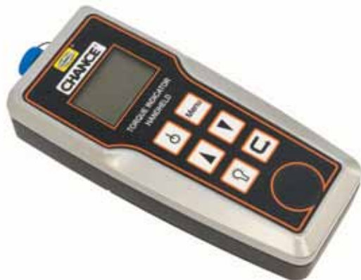
Remote Data Logger Figure 6-14
