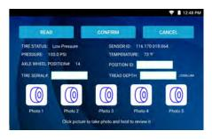
The **Equipment Walk Around** feature is a fast and easy way to capture and store tire pressure and temperature data for each vehicle. It's designed for the technician to to press and hold a tire location to transfer the tire pressure and temperature data for each wheel position.
