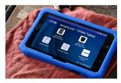
One-Click™ Transceiver to quickly access and record digital tire pressure and temperature data from Individual Sensor Readings, Equipment Walk Arounds or by transferring the data from the SmartLink™ One-Click™ Transceiver.
