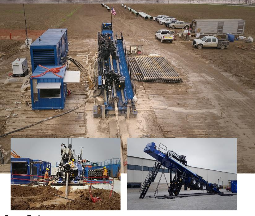
**Power Train** Engine: Cummins QSX15 Tier 4 Final **Rating:** 600 HP (447 kW) Fuel Capacity: 650 U.S. gallons (2,460 L) Hydraulic Capacity: 220 U.S. gallons (833 L) **Hydraulic Filter:** 6 Micron ABS Aux. Power Unit: Hatz 1B40 Diesel 9.9 HP (7.38 kW)
