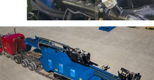
**Dimensions/Weights** Length: 52.5 ft. (19.05 m) Height: 11.5 ft. (3.5m) Width: 8.167 ft. (2.5 m) Transport Weight, Standard Configuration, w/o Wrenches: 75,368 lbs. (34,186 kg)
