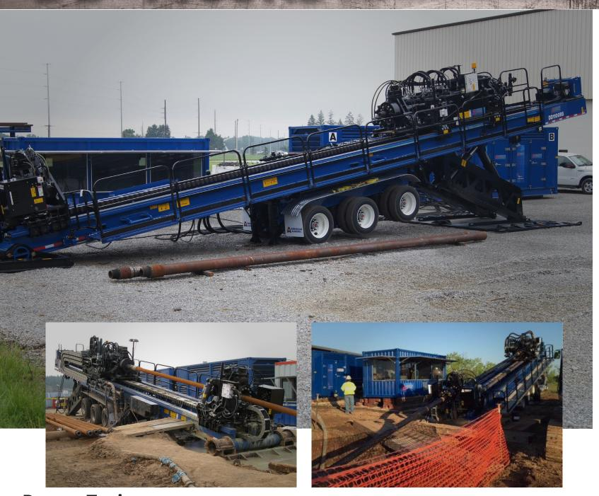
**Power Train** Engine: Caterpillar C-18 Tier 4 Final **Rating:** 755 HP (563 kW) Fuel Capacity: 650 U.S. gallons (2,460 L) Hydraulic Capacity: 220 U.S. gallons (833 L) Hydraulic Filter: 6 Micron ABS Aux. Power Unit: Hatz 1B40 Diesel 9.9 HP (7.38 kW)
