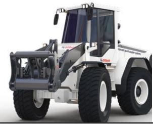
Change tools such as log forks, high dumping buckets, pallet forks with hydraulic tine adjustment, sweepers, bale clamps, and rotating bale clamps quickly from the comfort of the cab.
