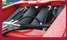
Robust, four-cylinder hydraulic removable gooseneck maximizes lift capacity and load height.
