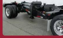
Allows users to operate as a 3+1 spread-axle with the E1Nitro™. Can also function as four axle close coupled.
