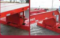
Sliding pin or swinging teardrop connections available for enhanced tractor compatibility.
