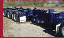
The E3Nitro™ is designed for trailers with up to 85-ton capacities and can carry 74,100 pounds in its 3+3 configuration.
