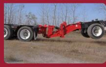
The E1Nitro™ is designed for trailers with up to 60-ton capacities and can carry 24,700 pounds in its 3+1 configuration.
