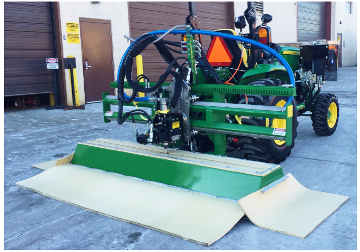
Thick, durable deflection mats keep debris contained.
