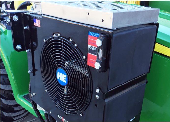
The 6600-3 uses a dedicated hydraulic system to run more efficiently and keep oil cooler.
