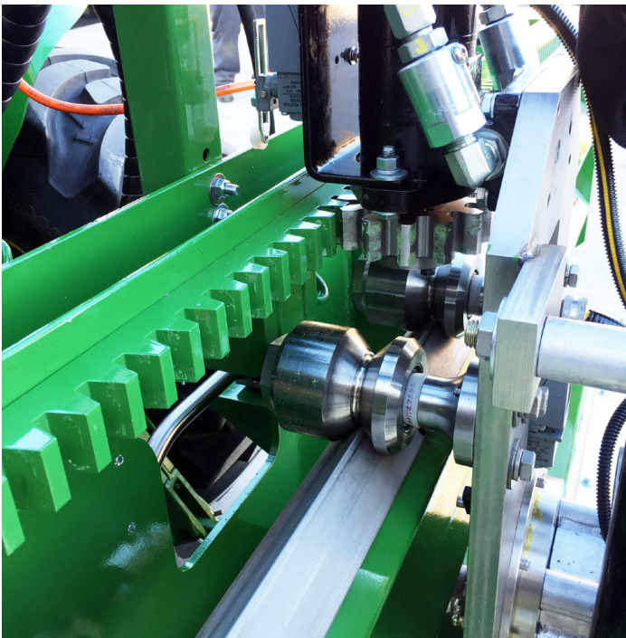
Traversing/oscillating removal head is adjustable for both removal depths and width of cut.
