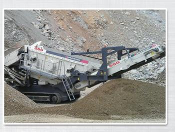
The high performance NFS550 is designed to work after a primary crusher or on its own as a frontline tracked mobile screening machine. NFS550 inclined screen is widely used in quarry, mine construction, waste of demolished building, surface soil, materials recycling, and screening of gravel, coal mine and aggregates. The plant has the capacity to process at a rate 500 t/h and can be fed either by a tracked mobile crusher or an excavator.
