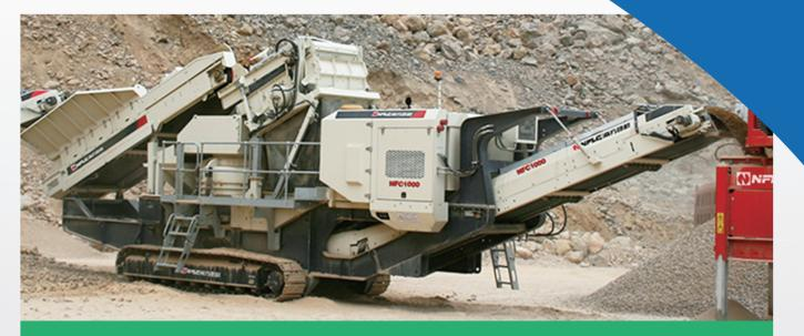
Hydraulic driven cone crushing host with adjusted speed and high yield can guarantee the finished product grain shape.
