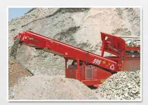
NFS150 is a self-contained high capacity mobile scalping unit. Designed and constructed to the highest specification, the NFS150 can withstand the toughest of applications from waste reclamation projects to quarry face and demolition environments, special features include a heavy duty twin deck vibrating grid, remote control movement.
