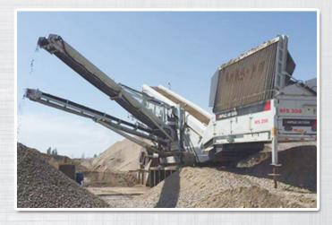
Renowned for its quality, performance and productivity the NFS330 combines scalping, screening and stockpiling into one self-contained unit. Its rugged design enables the NFS330 with its top deck 3.65m x 1.5m and bottom deck 3.00m x 1.52m screen to handle materials such as sand and gravel, limestone, crushed stone, coal, topsoil and demolition waste. Remote tipping reject grid, hydraulic screen tensioning of bottom deck mesh and three on-board hydraulic folding conveyors are standard.
