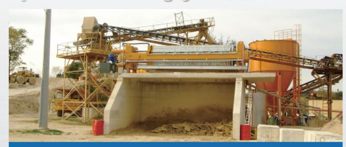
It allows to pump the slurry water collected in the agitating poolto itself to get treatment. Afterprocessing the slurry water is separated into solidified and hardened mud cake and clear water. The former one could be further processed and the later one is reclaimed to the agitating pool for further usage.
